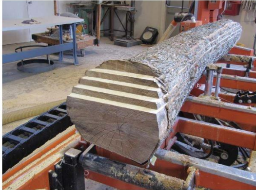
Figure 4.—Log being live sawn. Photo by Neal Bennett, U.S. Forest Service.
