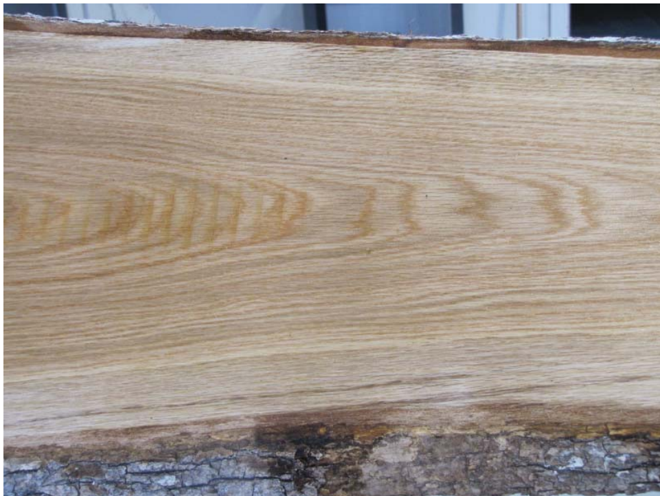
Figure 5.—Live sawn board showing varied grain pattern. Photo by Neal Bennett, U.S. Forest Service.
