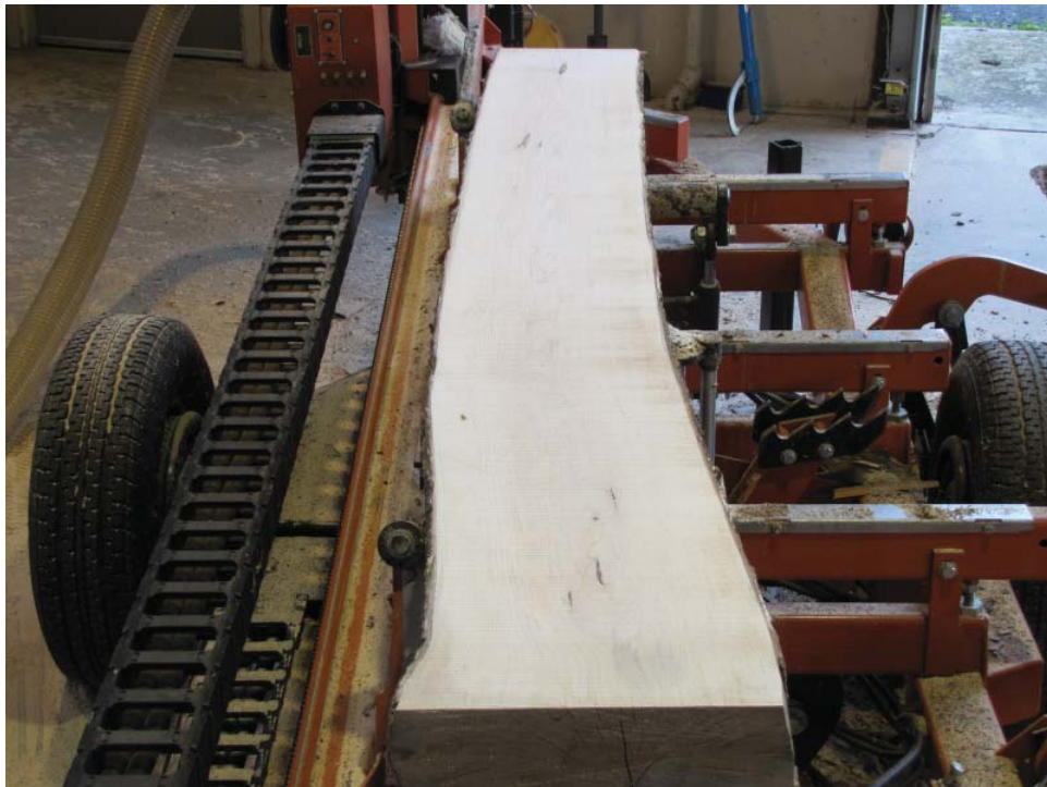
Figure 8.—Crooked board face from crooked live sawn log. Photo by Neal Bennett, U.S. Forest Service.
