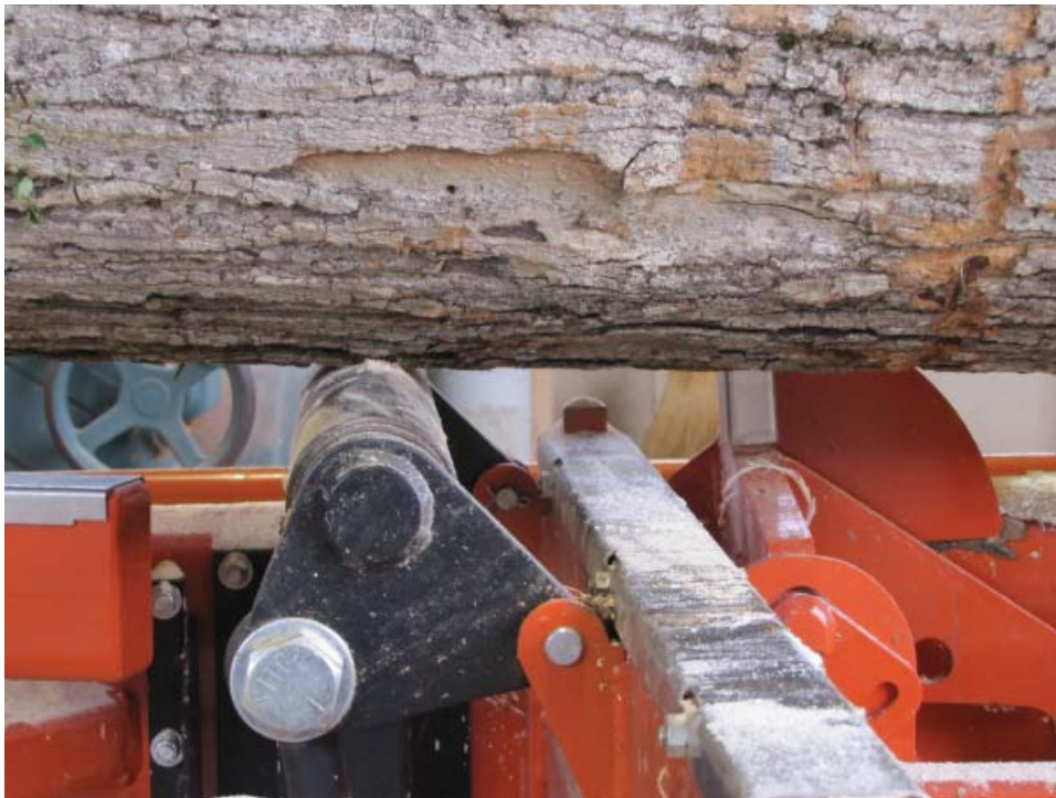
Figure 3.—Toe board leveling log parallel to the saw blade. Photo by Neal Bennett, U.S. Forest Service.
