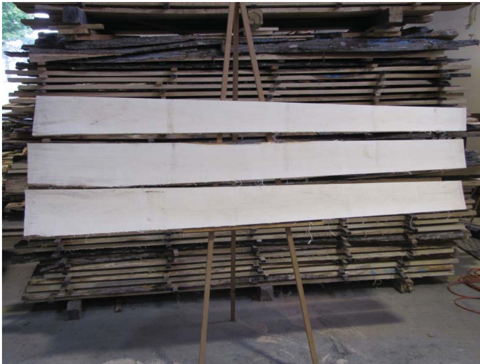
Figure 6.—Wedge shaped boards from taper sawn log. Photo by Neal Bennett, U.S. Forest Service.
